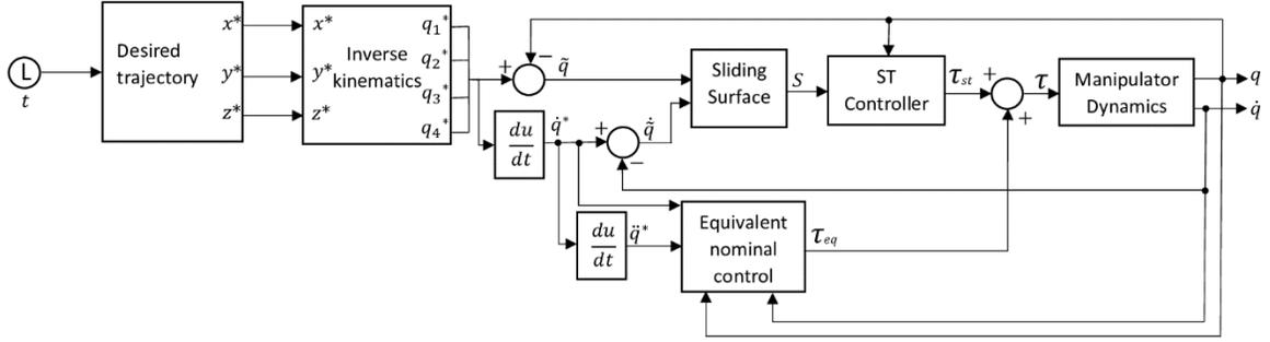
**Figure 6.** Block diagram of the STA controller.
