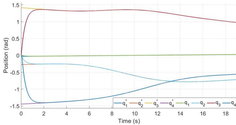
**Figure 12.** Trajectory tracking in joint space with ST.
