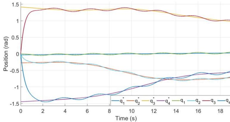
**Figure 11.** Trajectory tracking in joint space with PD+ Control.
