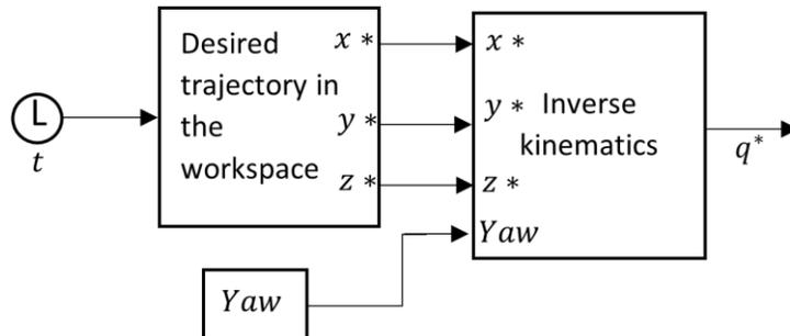
**Figure 10.** Scheme used to know the desired angles in each joint.
