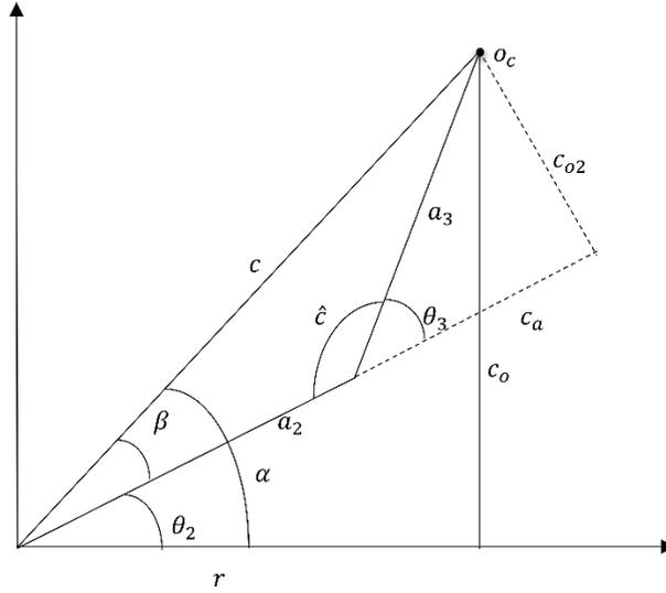
**Figure 8.** Position relation formed by the links  $a_2$  and  $a_3$  of the robot manipulator.
