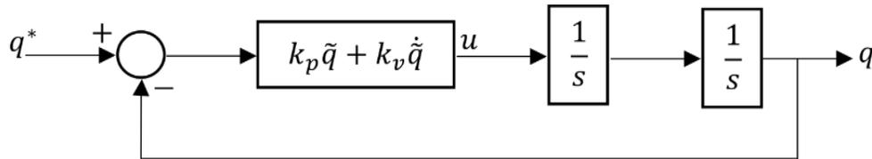
**Figure 4.** Block diagram of the linear system.
