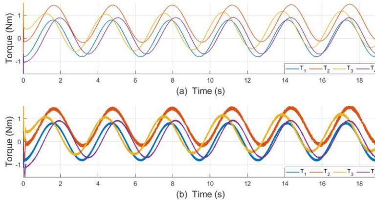
**Figure 13.** (a) Control actions of PD+; (b) Control Control actions of ST control.
