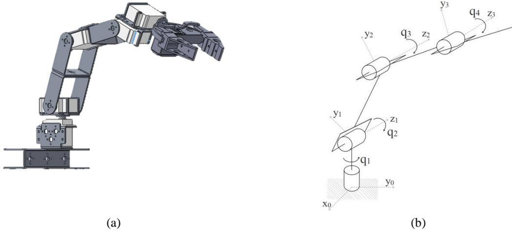
**Figure 2.** (a) Virtual model of the manipulator; (b) Coordinate frames attached to the manipulator.
