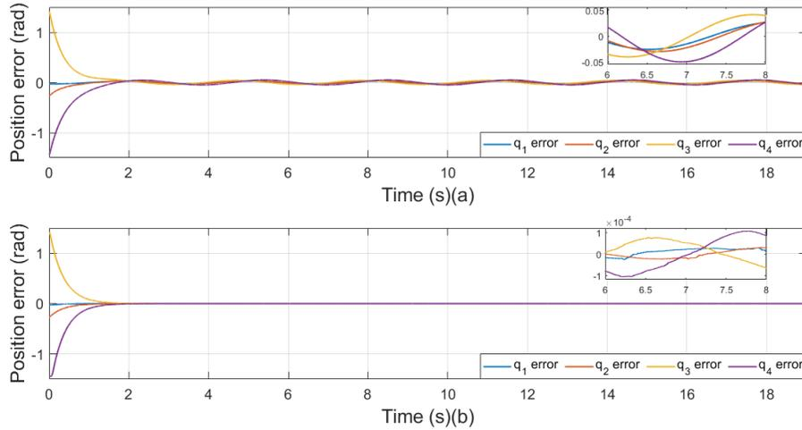
**Figure 14.** Position error in joint space with (a) PD+ Control; (b) ST Control.
