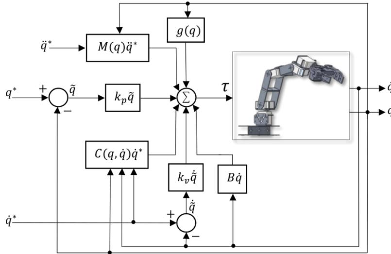
**Figure 3.** Block-diagram of the PD+ Control.
