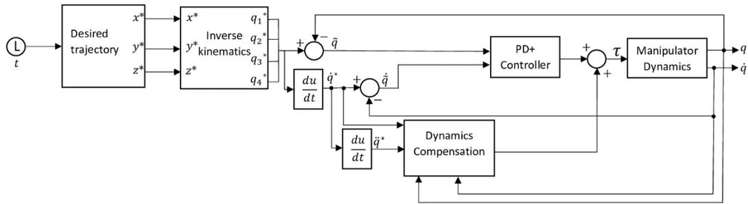
**Figure 5.** Block diagram of the PD+ Control for path tracking.
